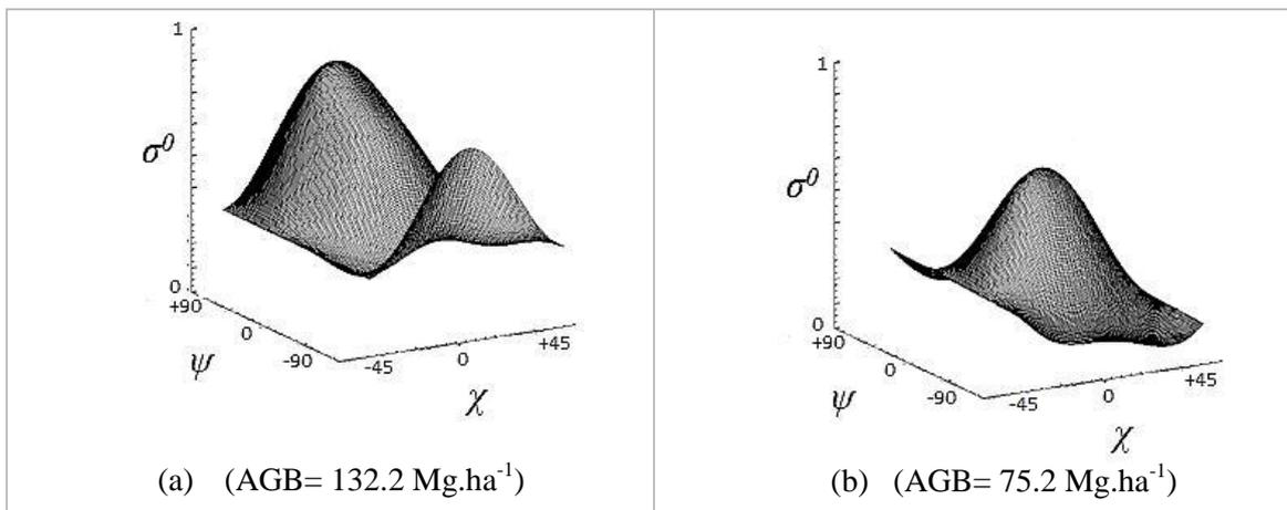
**Figure 1.** Polarization responses from PALSAR data over the forests affected once lightly burned (a) and thrice burned (b) in State of Roraima.
