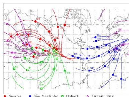
**Fig. 3:** The complete coverage of the GMDN - Global Muon Detector Network with the directions for each MMD's: Nagoya, Japan 17 directions; Hobart, Australia 13; Kuwait, Kuwait 13; So Martinho da Serra, RS, Brazil 17 (V, N, S, E, W, NE, NW, SE, SW, N2, S2, E2, W2, N3, S3, E3, W3).
