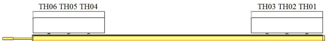
Figure 4. Position Monitoring Blocks in relation to Embedded Heat Pipe
