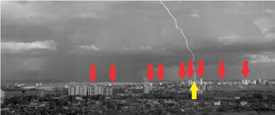
Figure 5 – Selected frame of a lightning flash registered by the R1 RAMMER sensor. The red arrows indicates the control points that were used for this case and the yellow arrow indicates the lightning stroke location in the image domain.
