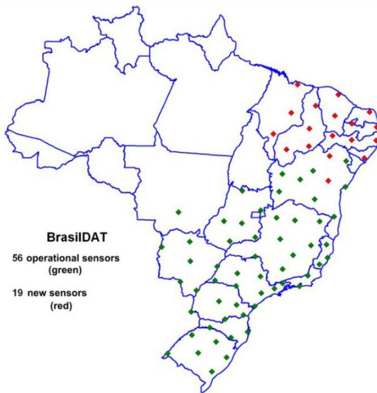
Figure 2 – Map of BrasilDAT sensors. The green diamonds represents sensors installed and operational and the red diamonds represents sensors that will be installed before the end of 2014.
