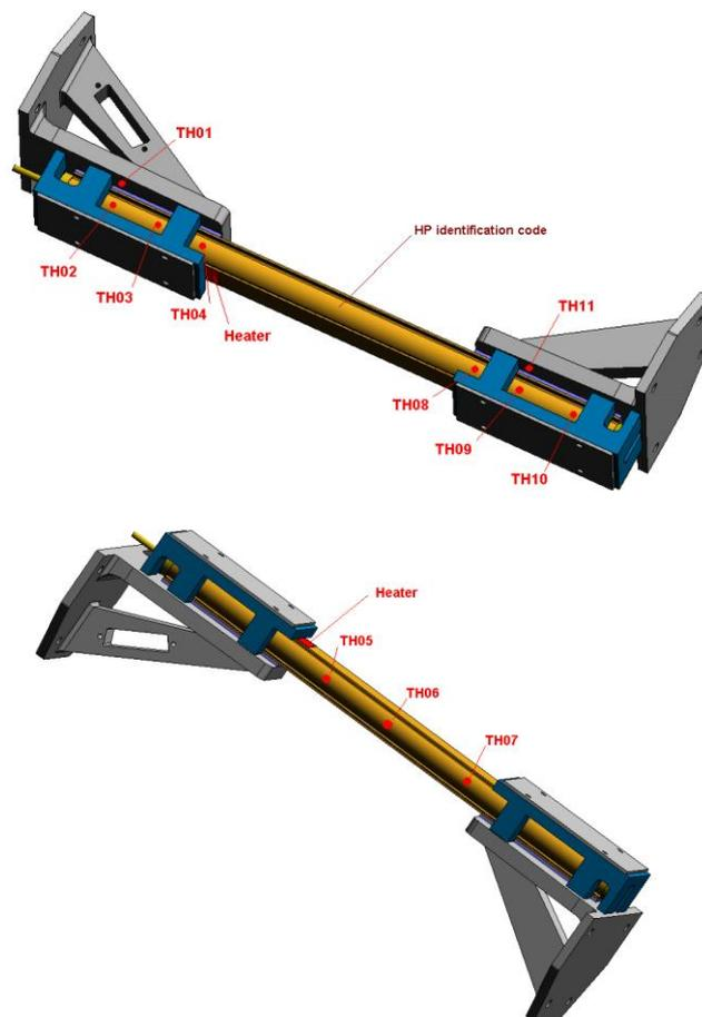
Figure 03- TUCA configuration (MLI and wiring are not shown).
