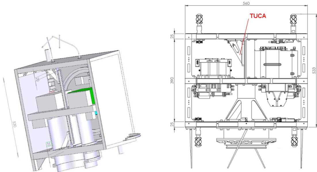
**Figure 02- (a) The ITASAT initial configuration and (b) actual modified version.**
