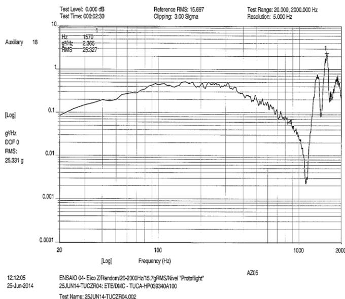
**Figure 15- Random-vibration test on the Z axis.**
