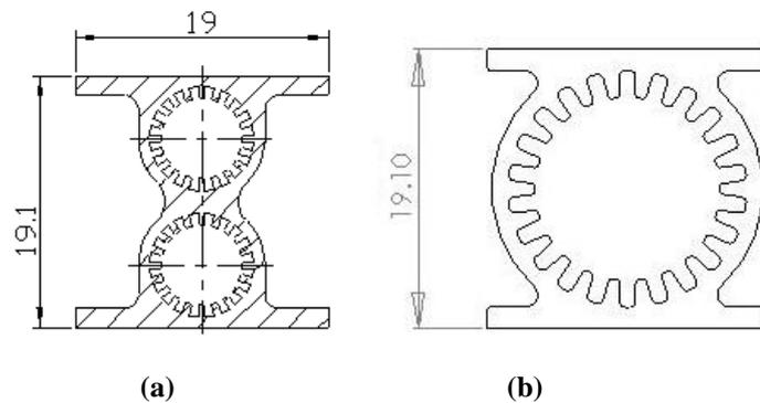
**Figure 01- (a) Inserted ammonia HPs that can be substituted by (b) acetone HP.**
