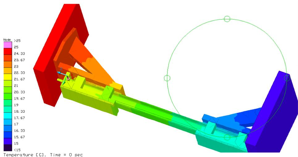
**Figure 05- Numerical simulation model that reproduced TUCA experimental using Thermal Desktop® SINDA/FLUINT.**
