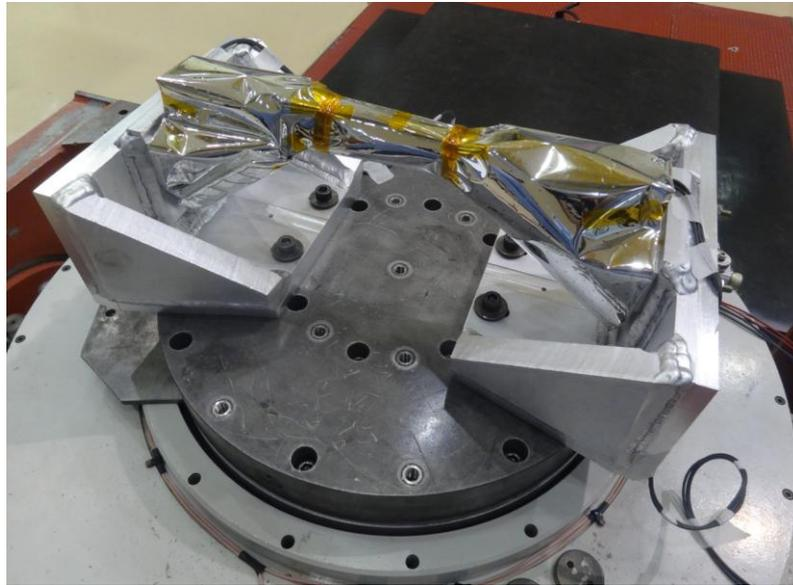
**Figure 13- TUCA under vibration test.**
