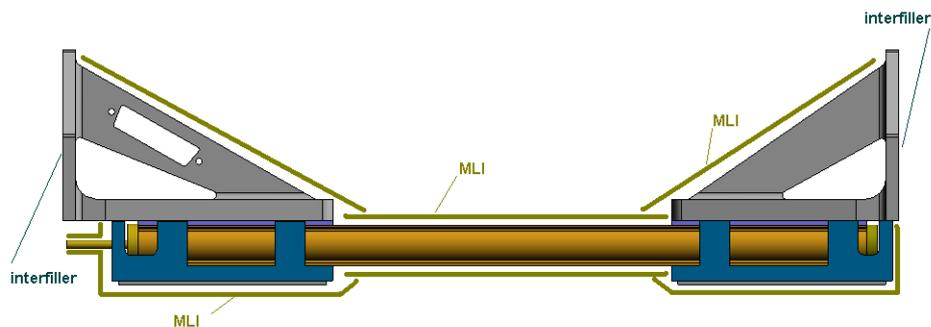
**Fig.04- MLI installation scheme.**
