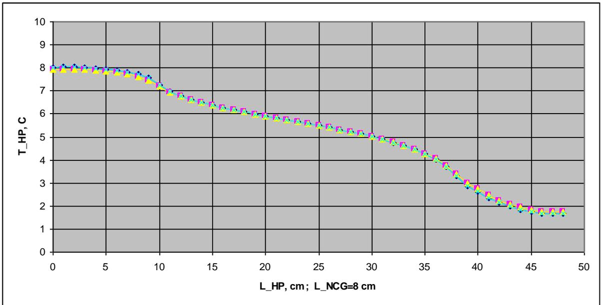
**Figure 11- Theoretical temperature profile indicates a presence of non-condensable gases with 8 cm.**
