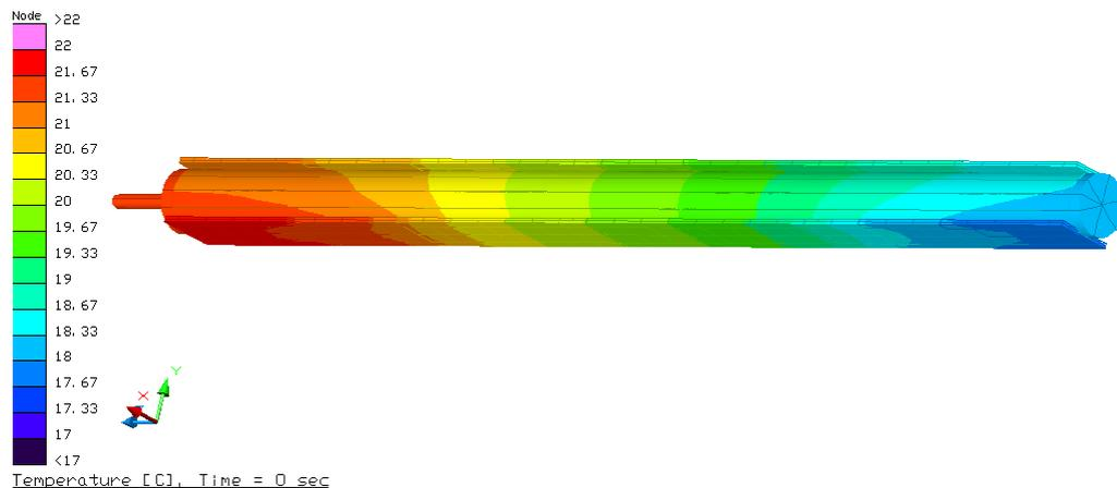
**Figure 06- Possible generation of non-condensable gases, blocking with 1 cm in the condenser of the heat pipe.**
