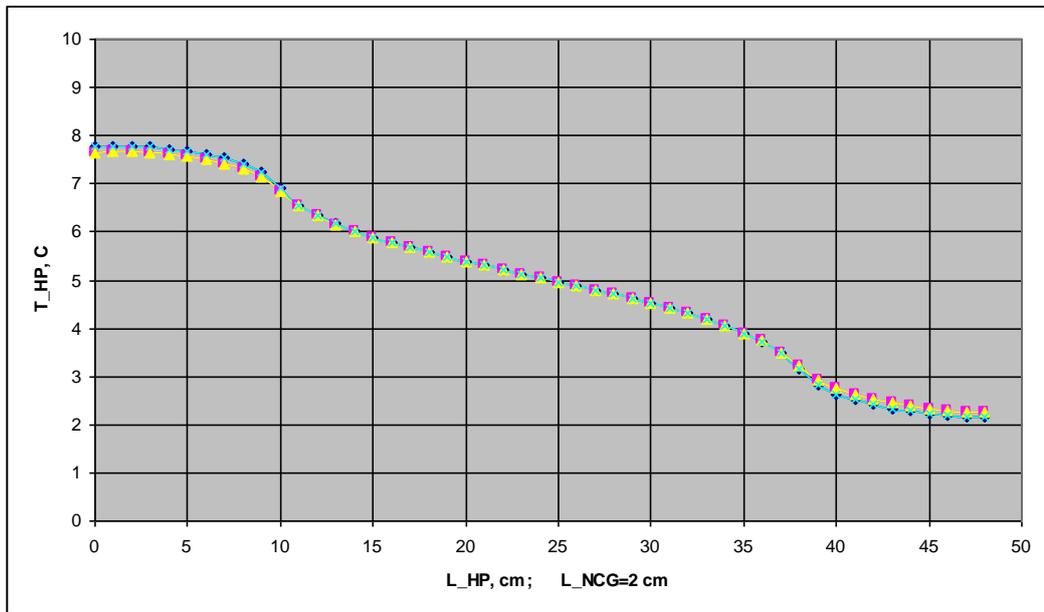
**Figure 10- Theoretical temperature profile indicates a presence of non-condensable gases with 2 cm.**
