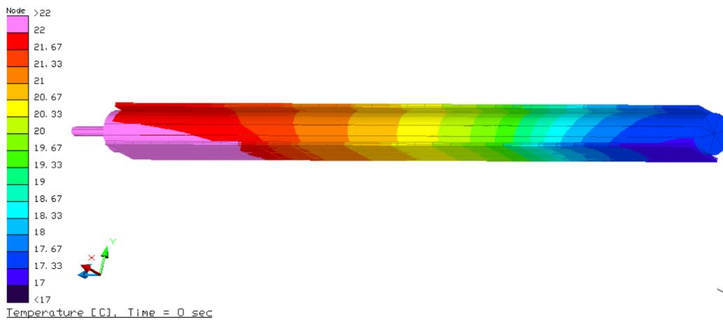
**Figure 08- Possible generation of non-condensable gases, blocking with 10 cm in the condenser of the heat pipe.**
