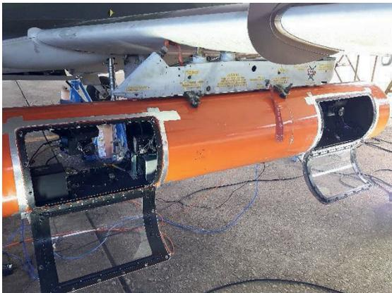
Fig. 3. Cameras installed and positioned inside the POD.
