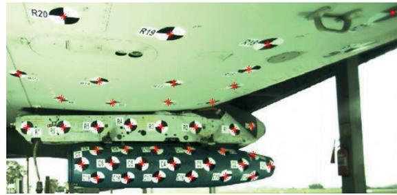
Fig. 12 Targets identified in store, pylon and wing.
