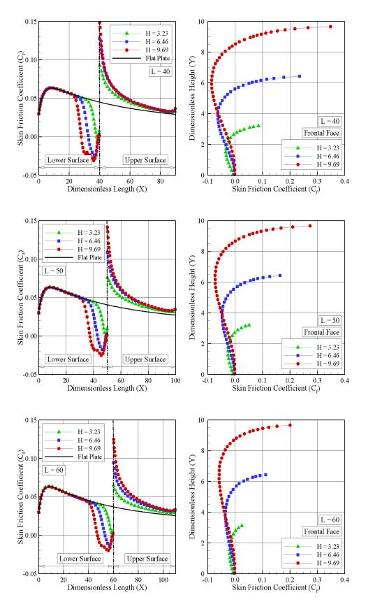
Figure 5. Distribution of skin friction coefficient  $C_f$  along lower and upper surfaces (left column) and frontal-face surface (right column) for dimensionless step position L of 40, 50, and 60.
