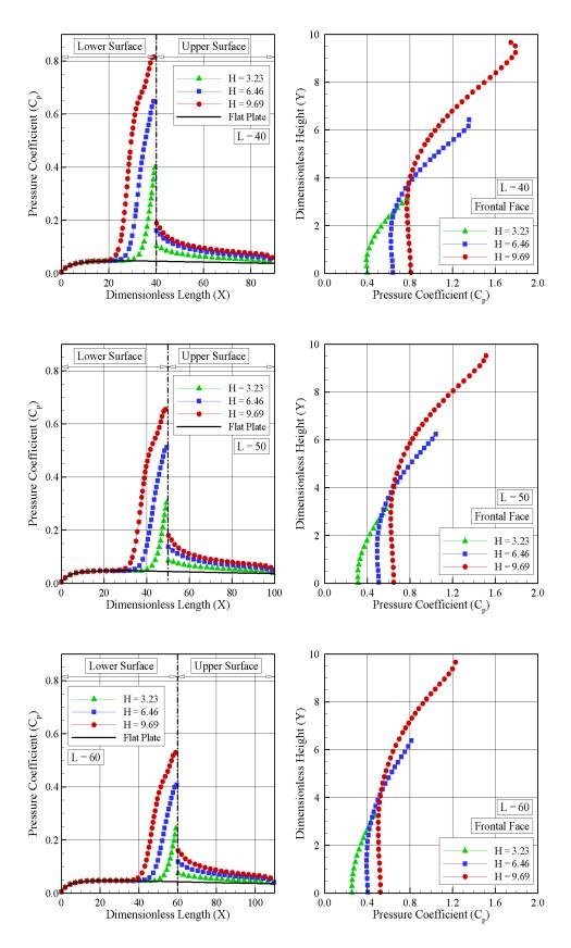
Figure 4. Distribution of pressure coefficient  $C_p$  along lower and upper surfaces (left column) and frontalface surface (right column) for dimensionless step position L of 40, 50, and 60.
