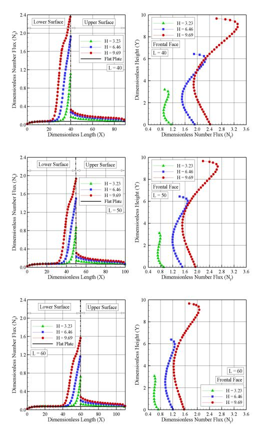
Figure 3. Distribution of dimensionless number flux  $N_f$  along lower and upper surfaces (left column) and frontal-face surface (right column) for dimensionless step position L of 40, 50, and 60.
