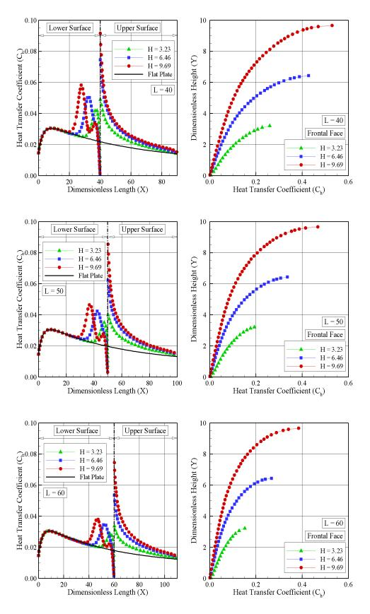
Figure 6. Distribution of heat transfer coefficient  $C_h$  along lower and upper surfaces (left column) and frontal-face surface (right column) for dimensionless step position L of 40, 50, and 60.
