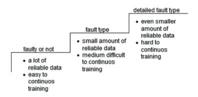
Figure 6: A stairway model for DGA Analysis
