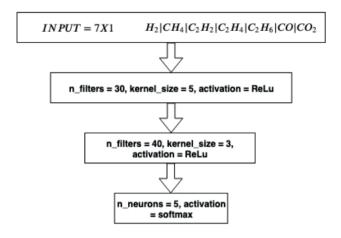
Figure 10. Convolutional Neural Network Topology
