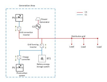
Fig. 4. Microgrid system legacy
