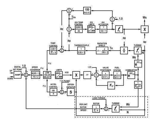
Figure 2. Model for CCPP applications (Yee et al., 2008)
