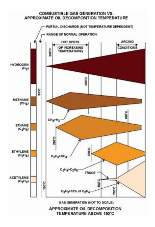
Figure 2: Faults and generated gases (Rogers, 1978)
