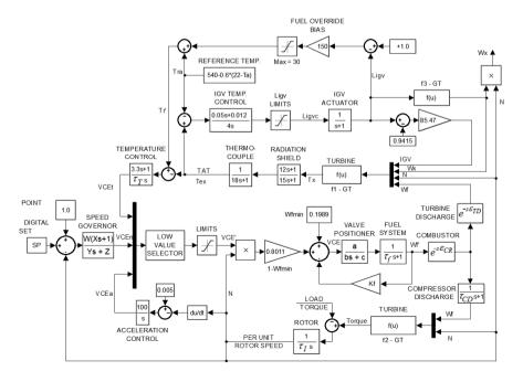
Figure 4. GT validated model in 'droop' mode with IGV control
