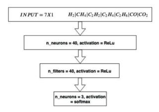
Figure 9: Multi-layer Perceptron Topology
