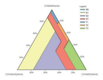
Figure 01: Duval Triangle 1 for DGA Analysis.
