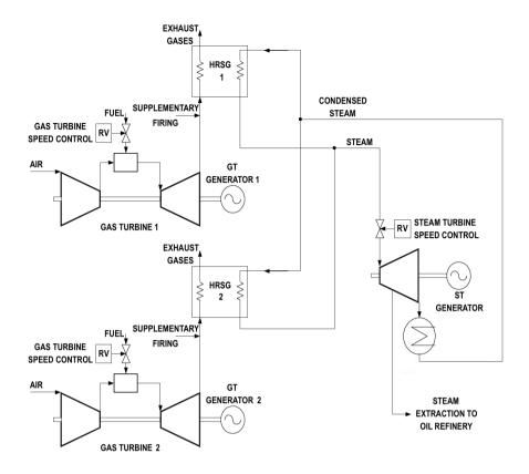
Figure 3. Schematic Diagram of Block I
