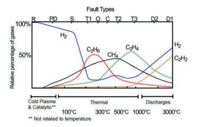
Figure 4. Faults and generated gases (CIGRE - JWGD1/A2.47, 2019)
