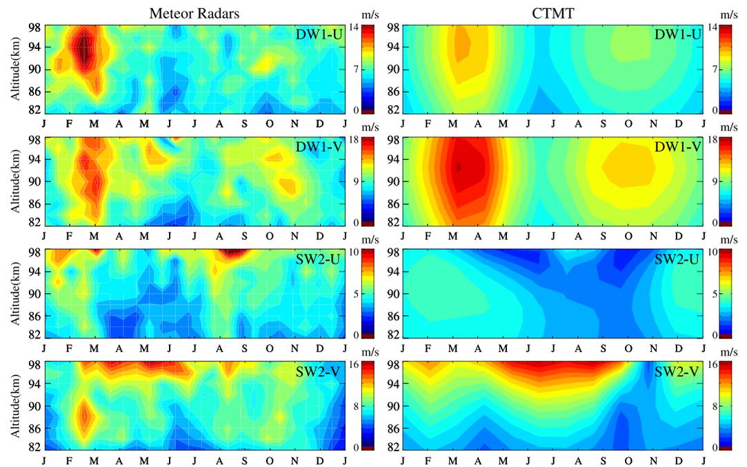
**Figure 8.** Meteor radar (MR) observations of the DW1 and SW2 tidal amplitudes in composite years in both wind components (in the left column) and the climatologies of the DW1 and SW2 tidal amplitudes derived from the Climatological Tidal Model of the Thermosphere (CTMT; in the right column). Different scales for the color bars show the different maxima of amplitudes for these tidal components.
