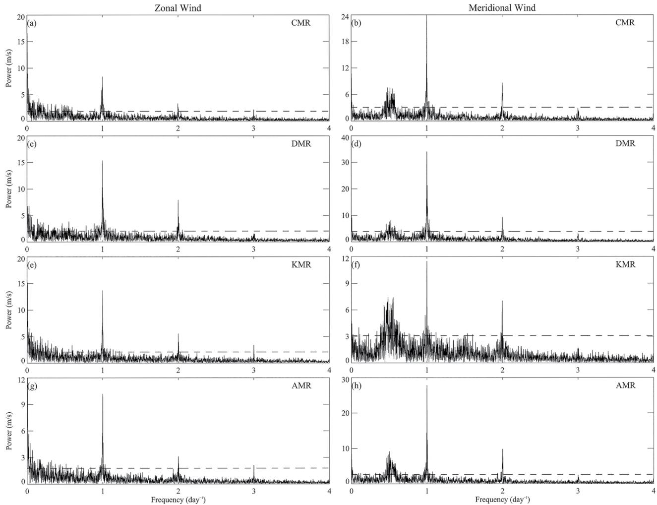
**Figure 2.** Lomb–Scargle analysis for the zonal and meridional winds observed by (a, b) CMR, (c, d) DMR, (e, f) KMR, and (g, h) AMR at 90 km. The black dashed lines represent the 95% significance level.
