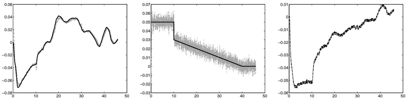
Figure 4. (Left) Estimation of the attack angle  $\hat{\alpha}$ . (Middle) Estimation of the bias  $\hat{b}_q$  at the  $q_L$  output. (Right) Estimation of the output  $\hat{\theta}$ . All sub-figures: grey lines - estimates, black lines - real variables; noise sources added to both plant outputs, with simultaneous occurrences of external disturbance and output bias (abrupt variation at 10 seconds).
