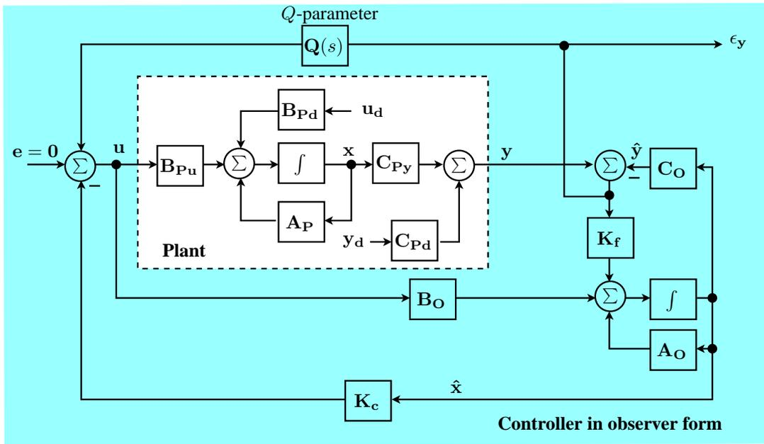
Figure 1. Observer-based structure using YOULA parametrization.
