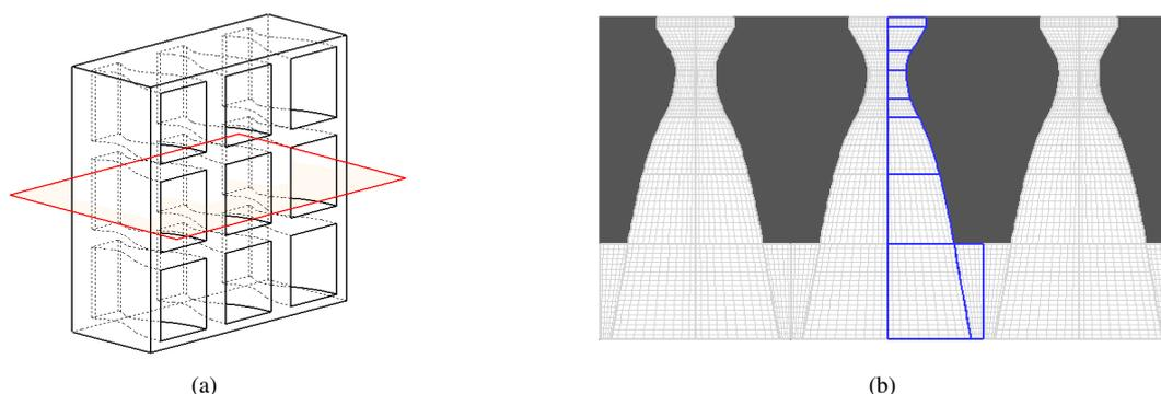
Figure 1. (a) Isometric view of a micronozzle array and (b) the two-dimensional representation of the simulated regions.
