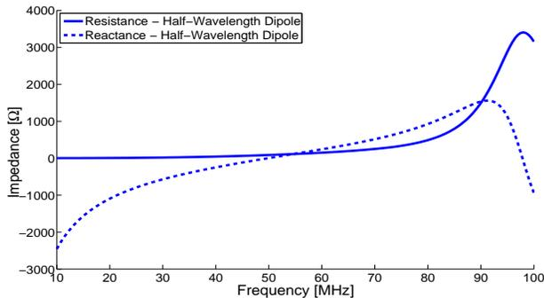
Figure 7: Simulated impedance characteristics for the Half-wavelength dipole.
