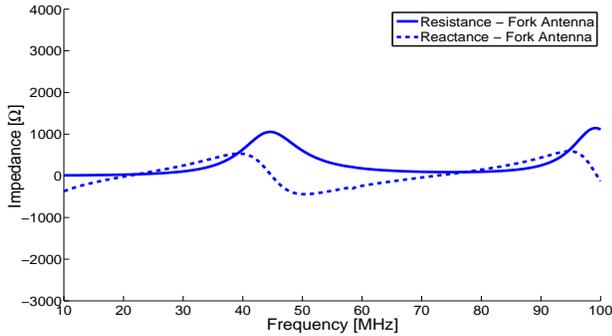
Figure 6: Simulated impedance characteristics for the Fork antenna.
