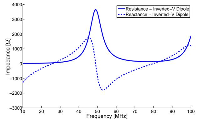
Figure 5: Simulated impedance characteristics for the Inverted-V dipole.
