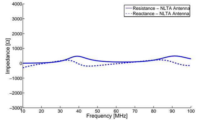
Figure 4: Simulated impedance characteristics for the NLTA antenna.
