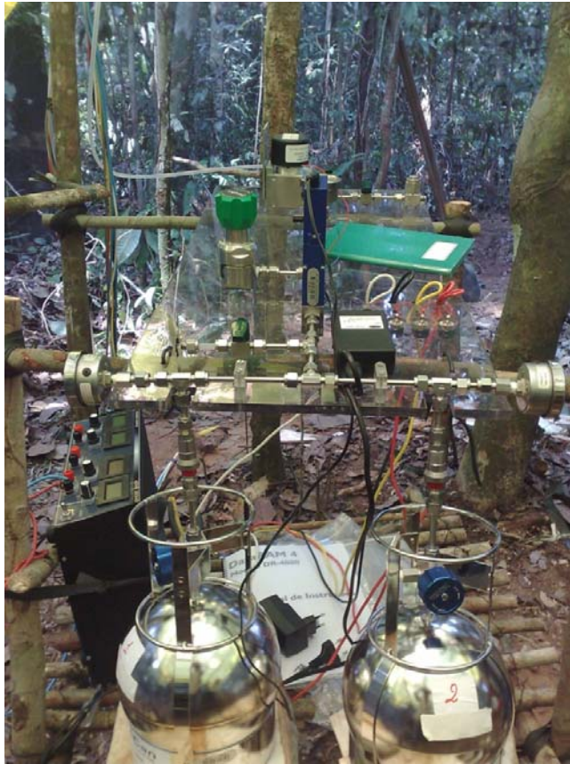
Figure 7 – Installation of system for field sampling.
