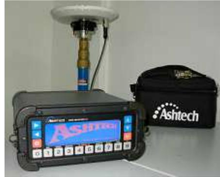
Figure 3 – Ashtech Z12 dual frequency GPS receiver
