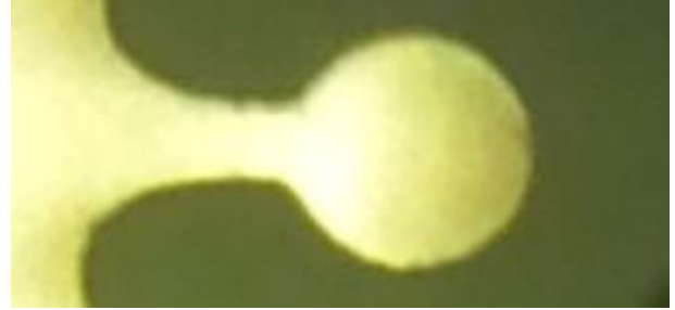
Fig. 7. Omega-type groove amplified view (a HP profile similar to one presented in [13]).
