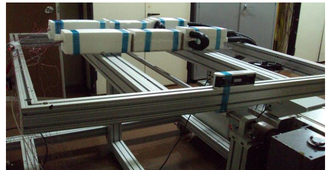
Fig. 17. Both heat pipes installed on the table.
