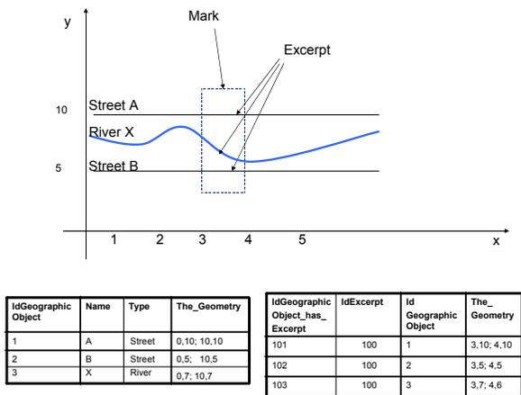
Figure 3. Example of the execution of the operation *boolean InsertAnnotation* (*Text* Annotation, *Geometry* Region, *Metadata* Metadata, *Context* Context).
