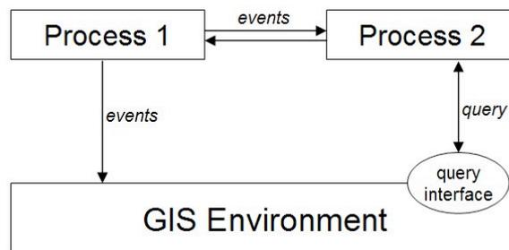
Figure 3. Two processes interacting with the GIS environment.
