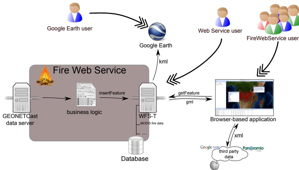
**Figure 3. Architecture of the Fire Web Service.**
