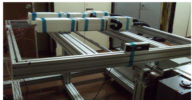
Figure 3. Both heat pipes installed on rotation table
