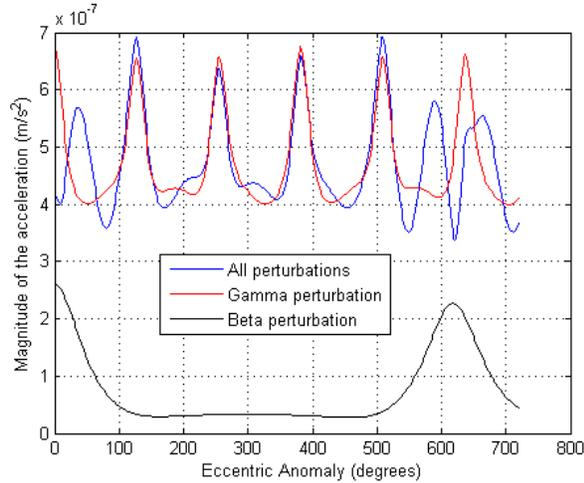
Fig. 10: The magnitude of the acceleration of the disturbing forces for two orbital periods.
