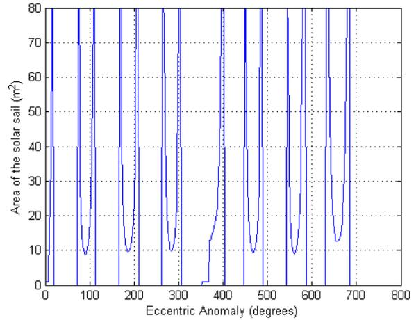
Fig. 13: The variable area of the solar sail for two orbital periods.
