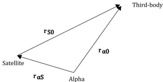
Fig. 2: Illustration of the third-body perturbation formulation.
