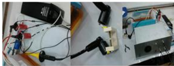
Fig. 2 – General view of the BD circuit, showing the ignition coil, the sample holder and the high voltage storage system.
