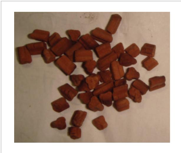
**Figure 1.**  $\text{Rh}_2\text{O}_3/\text{Al}_2\text{O}_3$  catalyst.
