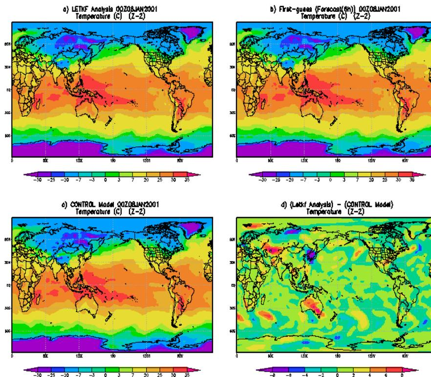
Fig. 2 Comparison of FSUGSM fields of temperature (°C) on sigma level 0.976 at 08/Jan/2001-00UTC, where (a) Letkf analysis field; (b) the forecast field; (c) control model field and (d) the differences field between analysis and control model.
