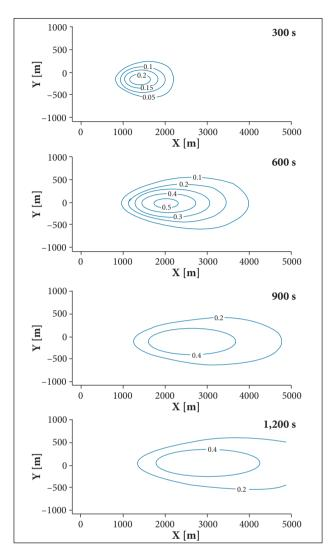
**Figure 8.** Isolines of concentration (mg/m<sup>3</sup>) at z = 1.5 m for Case 3 simulation.
