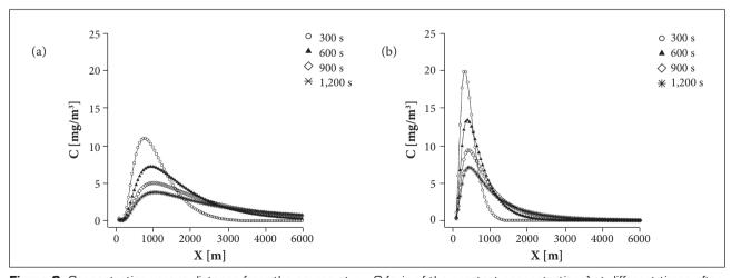
**Figure 6.** Concentration versus distance from the source at y = 0 (axis of the greatest concentrations) at different times after release for (a) Case 1 and (b) Case 4.
