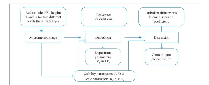
Figure 1. Flow-chart of the schematic model with the main features.
