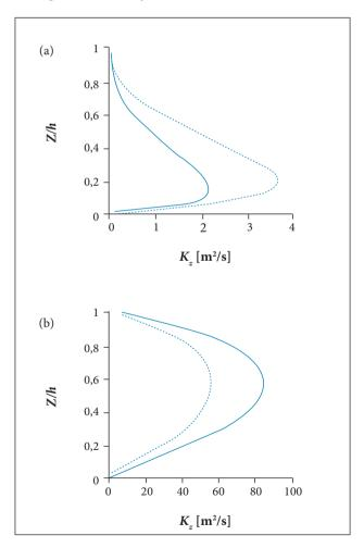
**Figure 2.** Vertical eddy diffusivities profile for (a) Stable cases – Case 2 (dotted line) and Case 3 (continuous line) — and for (b) Unstable cases – Case 1 (dotted line) and Case 4 (continuous line).
