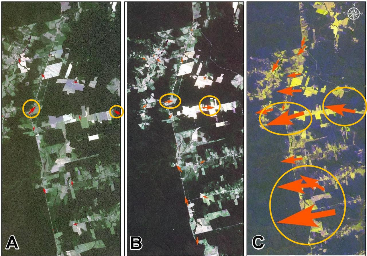
**Figure 6.** Arrows indicating the angular direction correction and proportion of the positional error for each set point for Spot- 6 images (A), RapidEye (B) and ResourceSat -1 (C). The orange circles indicate areas with larger errors in each image.
