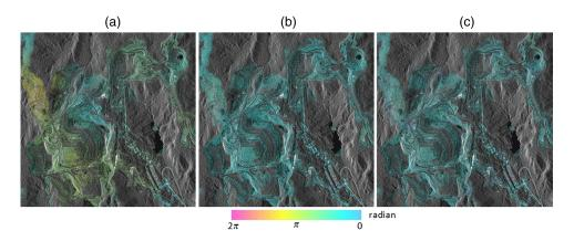
Fig. 6 Atmospheric residual phase components obtained after the (a) first iteration, (b) second iteration, and (c) third iteration for the pair of images acquired on October 4, 2012 (master) and October 28, 2012.
