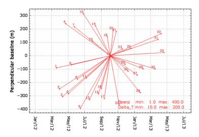
Fig. 5 Interferometric pairs in relation to the master image (October 4, 2012).
