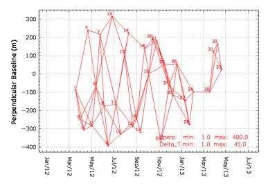
Fig. 3 Interferometric pairs selected based on the stack of 33 TSX-1 images, with constraints on time interval of 45 days and perpendicular baseline of 400 m.
