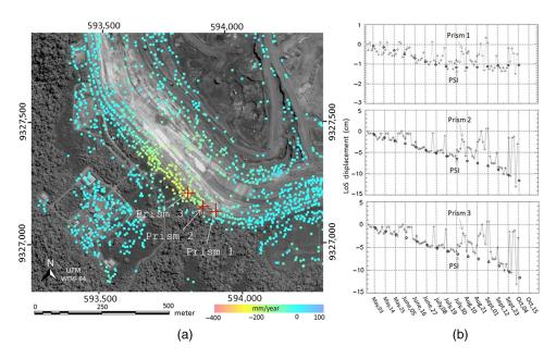
**Fig. 12** (a) Ground displacement map (LoS direction) of the slopes of N5W with prisms locations obtained from March 2012 to April 2013 and (b) the related displacement graphs (from May 3, 2012, up to October 4, 2012) for both techniques.
