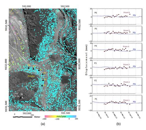
**Fig. 11** (a) Ground displacement map with six prims positions and (b) related graphs of displacement history for both techniques.
