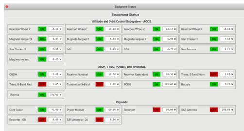
Figure 2: Equipment Module GUI [1]
