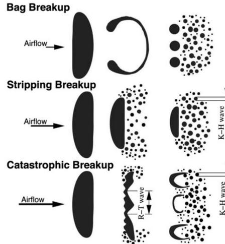
Droplets may suffer deformation and secondary atomization. A division according secondary atomization (Figure 2) based on experimental observations was reported and it seems to be dependent only on Weber number of the droplet (Faeth *et al.*, 1995).
