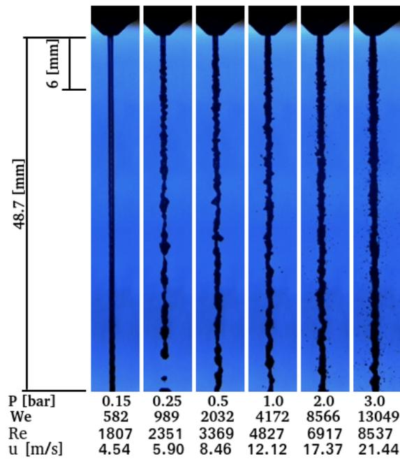
Figure 8. Hydrous ethanol sheet evolution with increasing of jet velocity,  $2\theta = 75^\circ$ .
