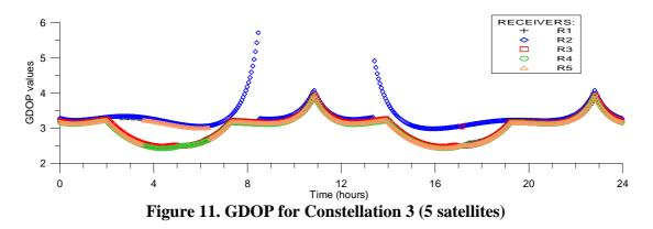
As can be seen from Fig. 11, there aren't peaks anymore in the GDOP values, and all five receivers have GDOP values under 6 during the entire propagation interval. The time percentages for GDOP < 4 is 100% for all receivers, but R2, that has GDOP < 4 during 94.9% of the time and GDOP < 5 during 99.1% of the time. These results corroborate the thesis that a fifth satellite in the Constellation 3 solves the GDOP peaks that occur when only 4 satellites are used.
