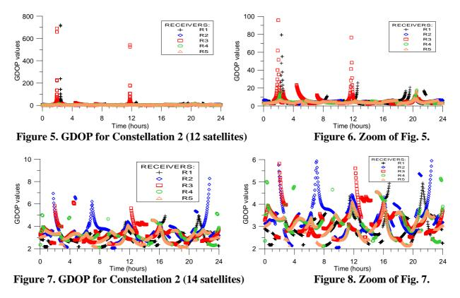
Figures 7 and 8 show that with 14 satellites the coverage is very good for all the receivers during the whole time, remaining below the value of 10 all the time and below 5 most of the time. The percentages of the time interval on which GDOP is less than 10 were 100.0% for all receivers. The percentages for GDOP < 5 were {100%; 93.4%; 98.1%; 99.1%; and 100%} for the receivers {R1, R2, R3, R4, and R5} respectively. In terms of computational time for Constellation 2, they
