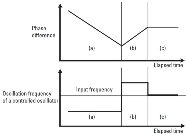
**Figure 7.** Phase difference and output frequency change over time during a phase synchronization process (digital control): (a) initial condition, (b) condition between the first and second digital controls, and (c) condition after the second control.
