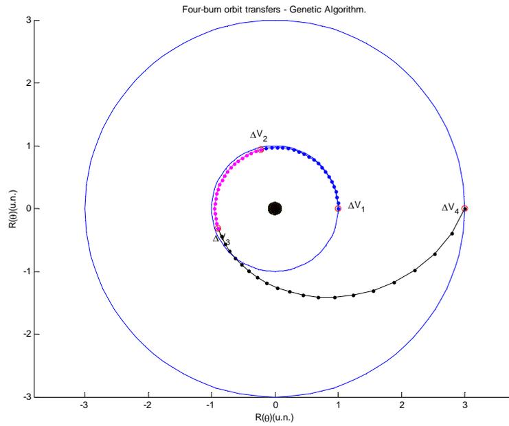
**Figure 3. Four-burn orbital rendezvous, simulation 2:  $r_0 = 1$ ,  $r_f = 3$ .**
