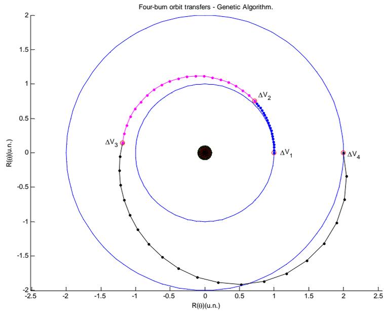
**Figure 2. Four-burn orbital rendezvous, simulation 1:  $r_0=1$ ,  $r_f=2$ .**
