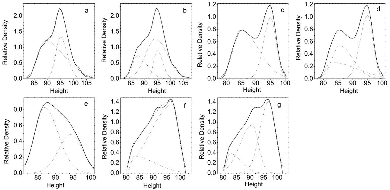
**Figure 5.** The improved background layer (solid curve) in case 1 is fitted by a layer (dashed curve), which is composed by (a) two Gaussians (dotted curves) and (b) three Gaussians. (c and d) As Figures 5a and 5b but for case 2, (e) as Figure 5a but for case 3, and (f and g) as for Figures 5a and 5b but for case 4.
