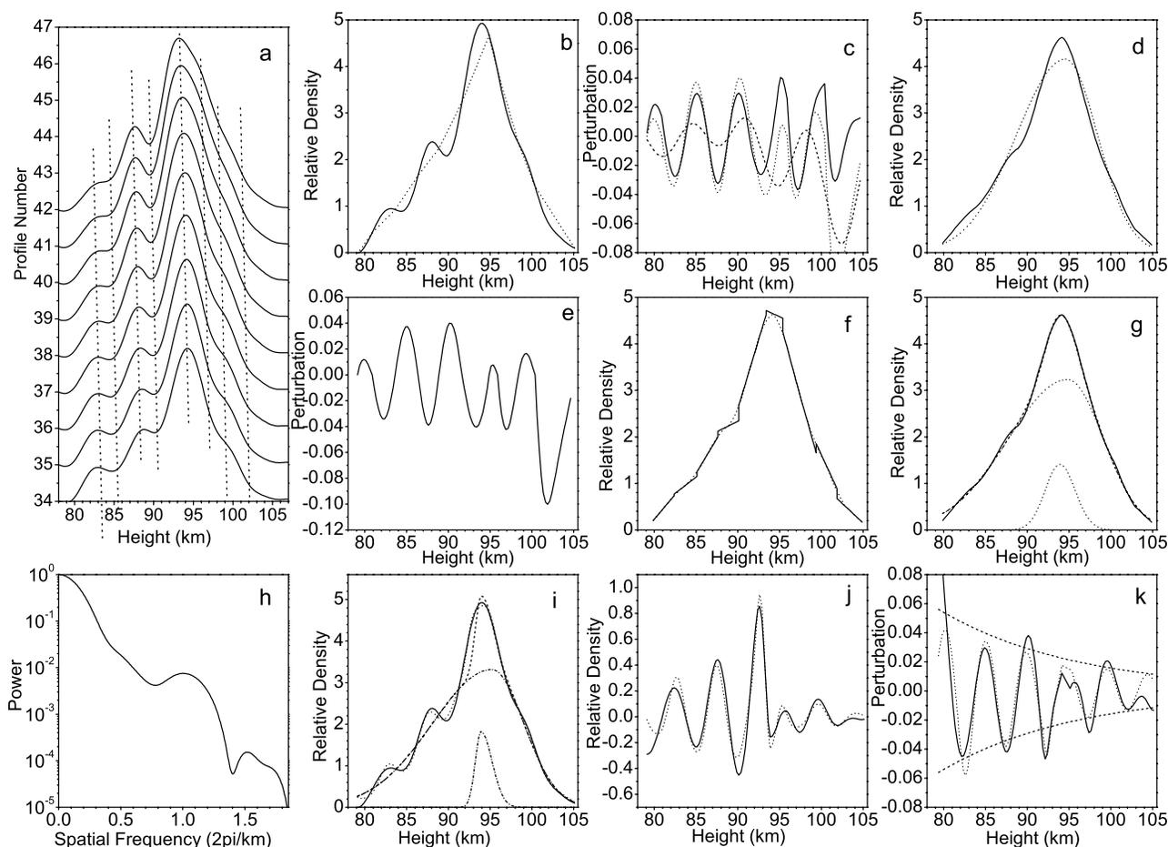
**Figure 9.** (a–k) The same as Figure 8 but for the observation example 2. The sodium lidar data sequence was observed on 4 June 1996 at São José dos Campos and the time interval between the profiles is 3 min.
