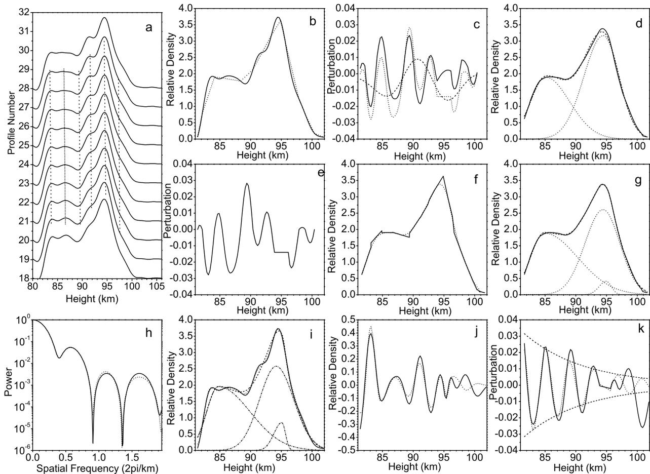
**Figure 12.** (a–k) The same as Figure 8 (except for Figure 12h) but for the observation example 5. Figure 12h shows the normalized power spectrum (solid curve) for the observed layer in Figure 12b and the spectrum (dotted curve) for the simulated layer in Figure 12i. The sodium lidar data sequence was observed on 21 October 1998 at São José dos Campos, and the time interval between the profiles is 3 min.
