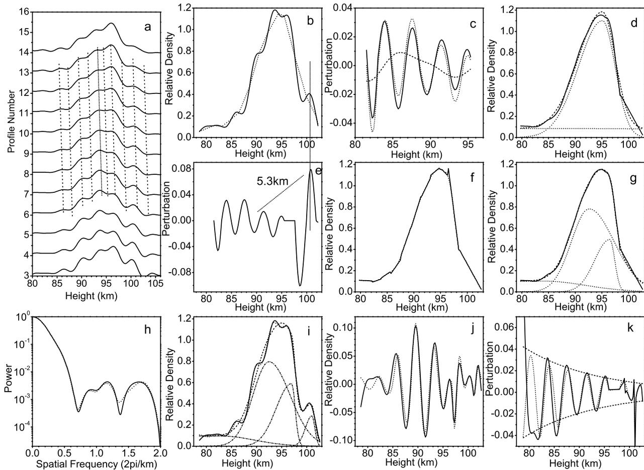
**Figure 11.** (a–k) The same as Figure 8 (except for Figure 11h) but for the observation example 4. Figure 11h shows the normalized power spectrum (solid curve) for the observed layer in Figure 11b and the spectrum (dotted curve) for the simulated layer in Figure 11i. The sodium lidar data sequence was observed on 17 November 2004 at Wuhan, and the time interval between the profiles is 3 min.
