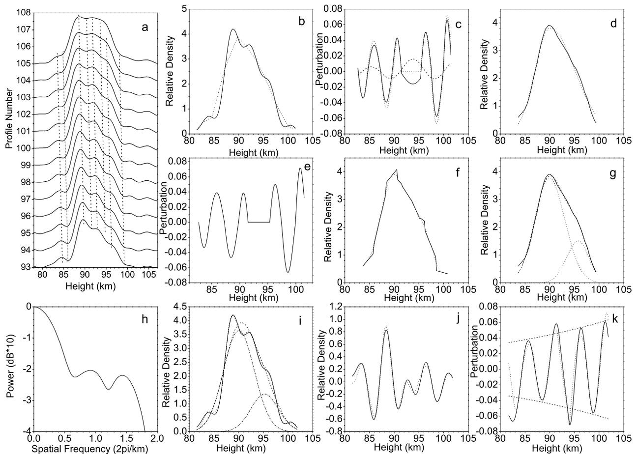
**Figure 13.** (a–k) The same as Figure 8 but for the observation example 6. The sodium lidar data sequence was observed on 17 November 1999 at São José dos Campos, and the time interval between the profiles is 3 min.
