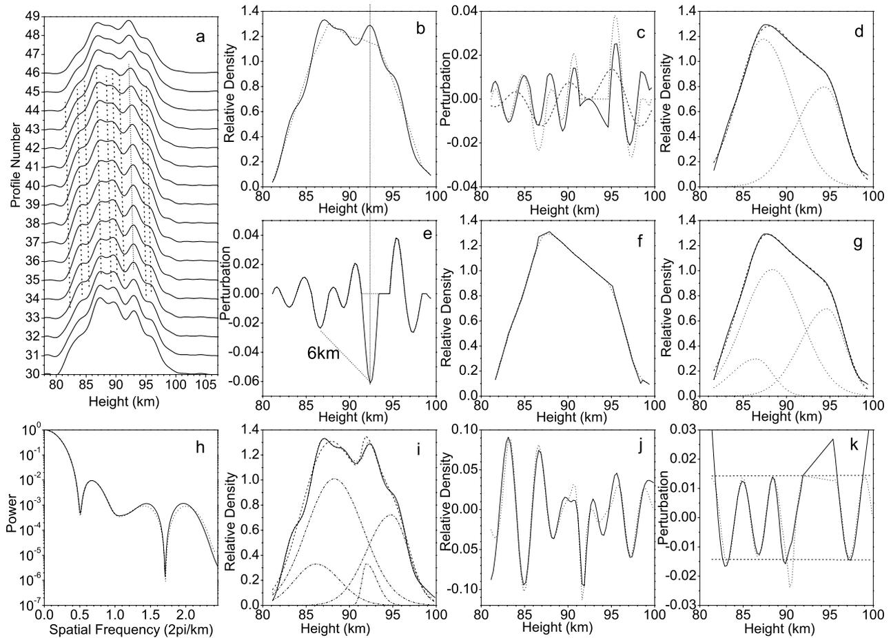
**Figure 10.** (a–k) The same as Figure 8 (except for Figure 10h) but for the observation example 3. Figure 10h shows the normalized power spectrum (solid curve) for the observed layer in Figure 10b and the spectrum (dotted curve) for the simulated layer in Figure 10i. The sodium lidar data sequence was observed on 1 December 1999 at São José dos Campos, and the time interval between the profiles is 3 min.
