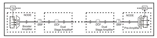
Fig. 8. General link architecture considered in our tests.
