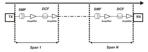
Fig. 1. Transmission system multi-span with dispersion compensation
