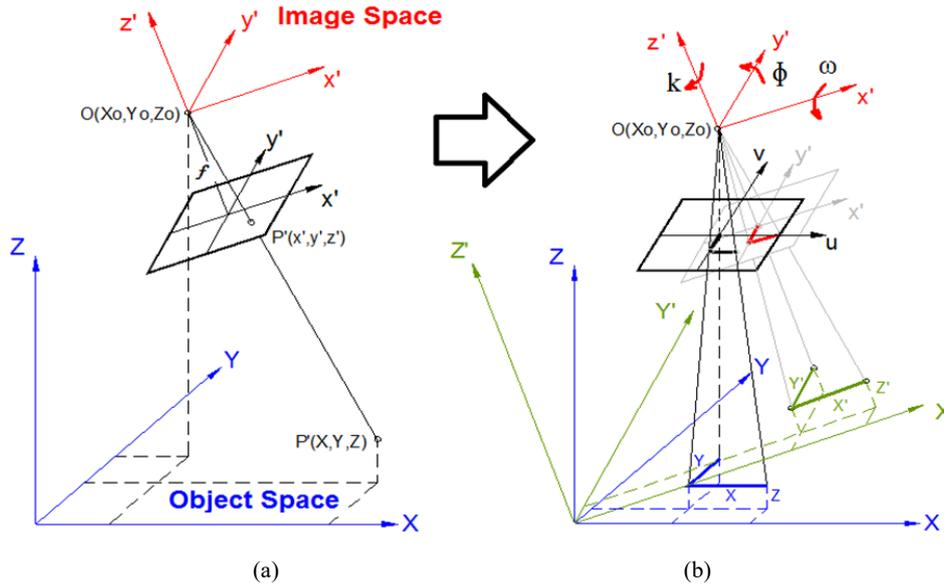
Fig. 1 Collinearity between Object Space and Image Space
