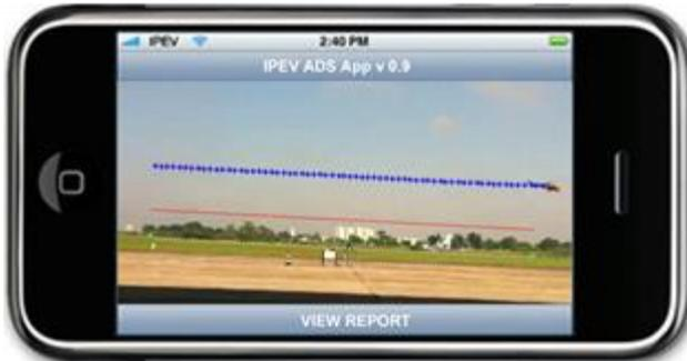
**Figure 4 – Superimposed marks of the aircraft trajectory, after the execution of a TP**
