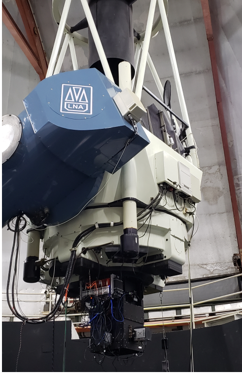
FIGURE 3. SPARC4 mounted in the 1.6-m telescope of OPD just before the first light on Nov 4, 2022.
