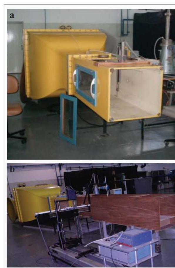
Figure 3: The wind tunnel (a) and an overview of the wind tunnel with the woody extension (b).
