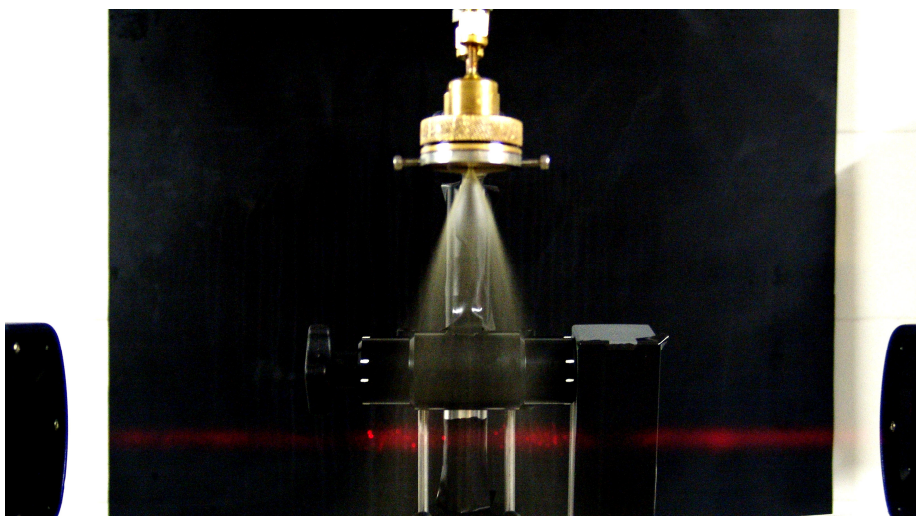
Figure 2. View of the injector with the laser beam emitted from the Spraytec laser system.
