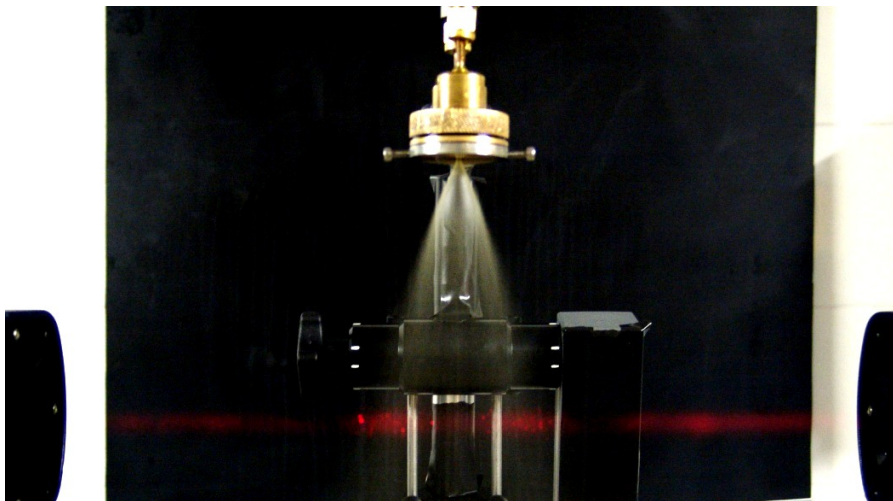
Figure 2. View of the injector with the laser beam emitted from a laser diffraction system (Spraytec).
