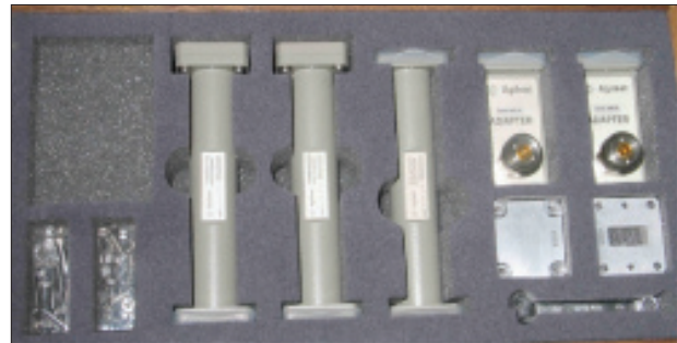
Figure 3: Waveguide calibration set for X band.
