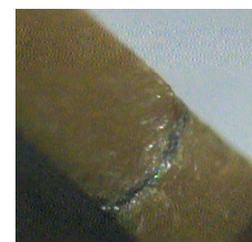
Fig. 9. Flashover channel formed on the capacitor 2 border.
