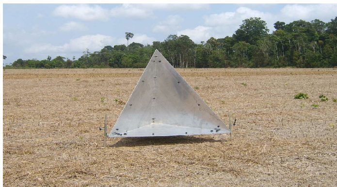
Figure 6. Corner reflector deployed in the Tapajós area.
