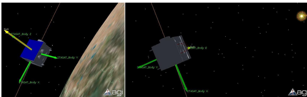
Figure 4. ITASAT sun-aligned body-fixed attitude coordinate frame
