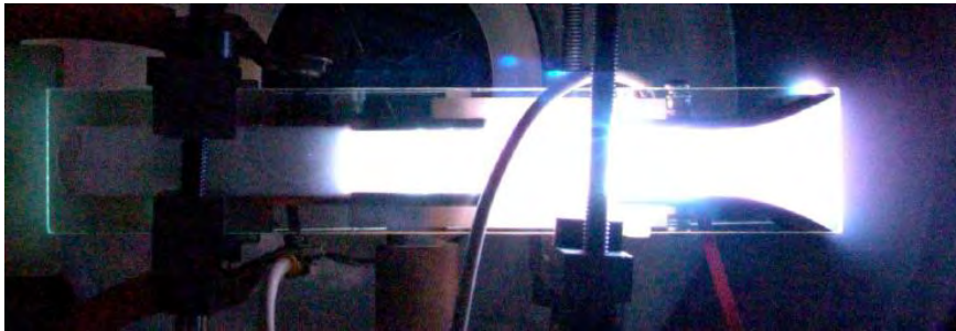
Figure 5: Laboratory DD-PPT plume.
