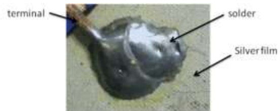
Figure 7. Cooper terminal firmly soldered to the PZT metallic electrode with no cracks or film release.
