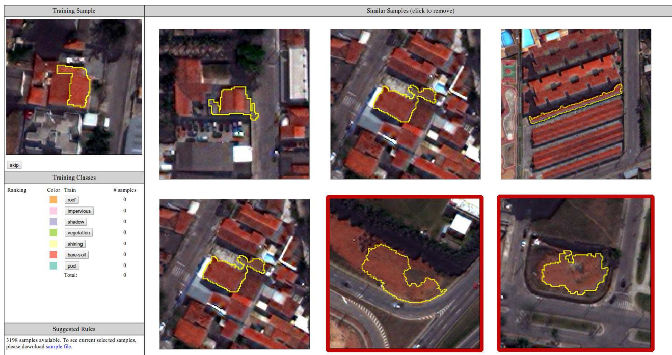
Figure 5. The GUI showing a target segment (on the left, marked as Training Sample ) and candidates to be included in the sample selection. The misclassified candidates are highlighted in red .
