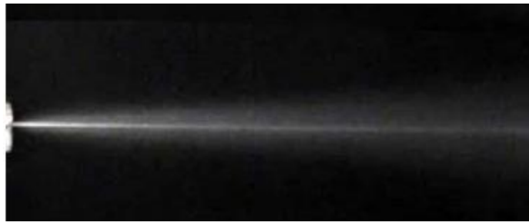
Figure 3 - Jet of liquid in the spray center line for ALR values below the minimum limit presented in Table 1. Azevedo (2013)
