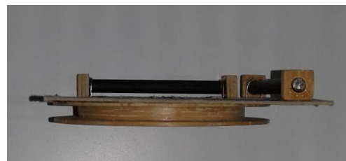
Figure 10 - Torquers and their ADCM board layout.
