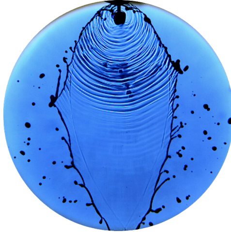
Figure 1. Hydrous ethanol liquid sheet, 2\theta = 90^\circ , u = 3.5 m/s
