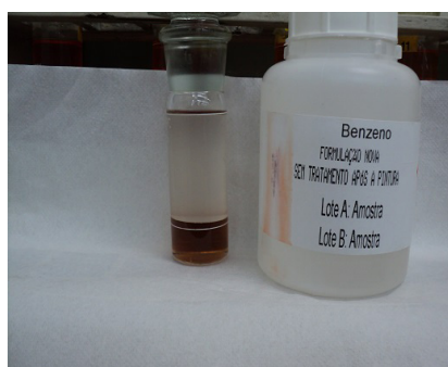
Figure 6. TS painted with Formulation 1, immersed in benzene; off-spec result ( > 1+ )
