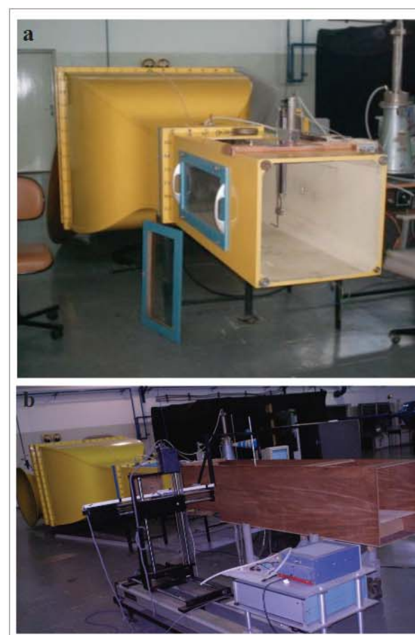
Figure 3: The wind tunnel (a) and an overview of the wind tunnel with the woody extension (b).
