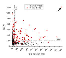
Figure 4. Scatterplot of the estimated peak current, Ip, versus CC duration.
